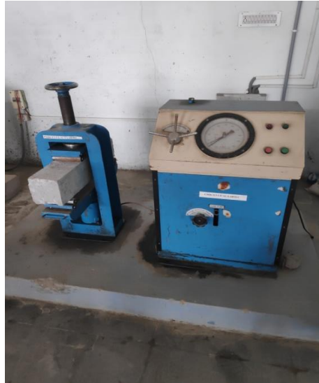
Fig 4.5: Flexural strength testing machine
