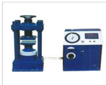
Fig 4.4: Sample testing on CTM for Split tensile Strength
