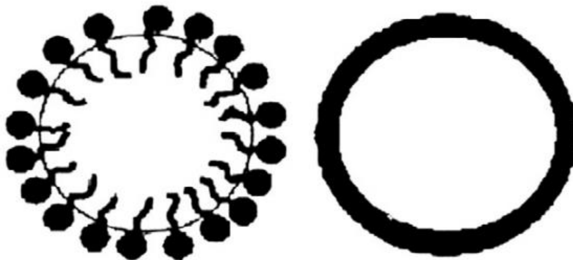
Figure 2: Illustrates the (a) nano emulsion and (b) biopolymeric nanoparticle[5].
