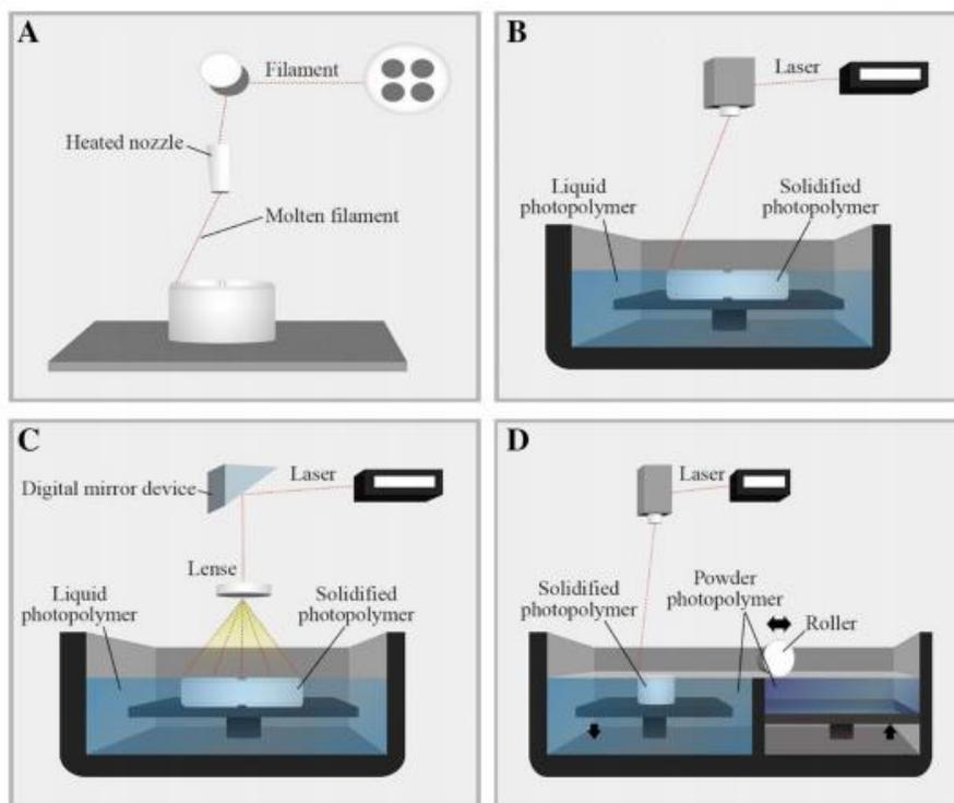
**Figure 1: Illustrates the Graphical illustrations of 3DP processes. (A) FDM printer (B) SLA printer (C) DLP printer (D) SLS printer [3]**
